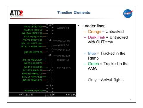
Leader lines are useful for determining the status/position of the flight on the surface.
