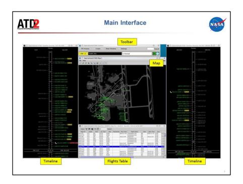
The full interface of the STBO Client is composed of multiple display windows that all serve different purposes and can be configured and arranged however the user wants.
