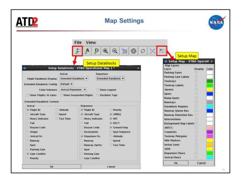
The Setup Datablocks button on the Map toolbar opens a window that enables changing the settings for what items are displayed on arrival and departure datablocks, as well as setting up how aircraft icons are color coded, showing (untracked) flights at the gate, and other display filters.
