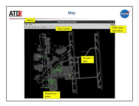
STBO Client Map consists of dropdown menus (which will not be covered in these slides since most of the functions are found elsewhere on the GUI), a Map toolbar, STBO Client Help menu, and flight positions on the surface. Flight positions are collected from surface surveillance.
