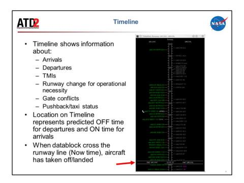
The Timeline is set up to display flight positions, resource labels (e.g., "18C/36C") at the top and bottom of the display, the type of resource (e.g., "Runway" at the top of the timeline or "RWY" at the bottom), and the now time. The timeline also provides information about arrivals, departures, TMIs, runway assignments and changes for operational necessity, gate conflicts, and pushback and taxi status.
